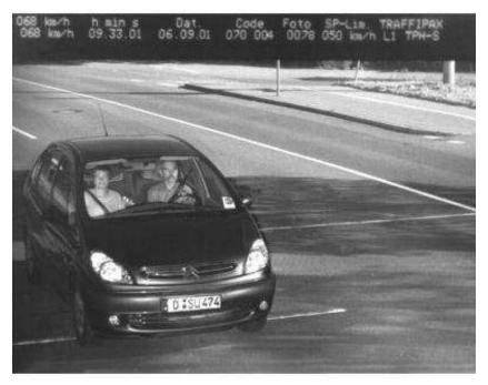
Meta data: Speed, when, where, photo ID, last calibration, ...
